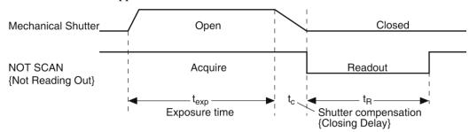
Figure 22. Exposure of the CCD with Shutter Compensation
